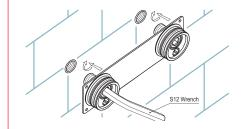
Wrap the two S-connectors with Teflon tape and put them through the locating plate and screw them into the pipe joint. Tighten them with S12 wrench (Fig.5 and Fig.6)
